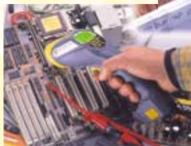
◀ Detection of hot point
