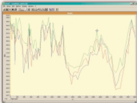
Representation of changes measured in the electric field along a covered distance is carried out in real time on 1 to 3 frequencies simultaneously
